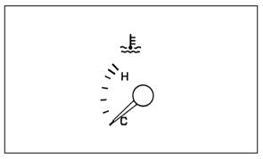
The engine coolant temperature gauge
